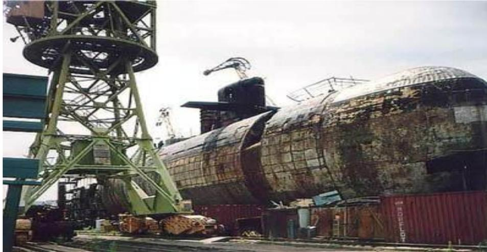
The CTR Programme Provided Equipment to Dismantle Russian Ballistic Missile Submarines<sup>8</sup>
